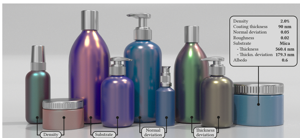
Fig. 1. We present a general model for pearlescent materials, which simulates their complex optical behavior. Our model reproduces and parameterizes the key physical attributes produced by the manufacturing process of such materials, and the resulting reflectance functions closely agree with measured data. In this image, we show how changing a single parameter in each pair of bottles (as indicated by the brackets) leads to large, difficult-to-predict changes in appearance. From left to right, the changed parameters are: a) platelet density variation; b) substrate composition; c) deviation of the platelet normal distribution; d) deviation of the substrate thickness. The rightmost jar shows the values of our model parameters for its particular material. Please refer to Table A3 for a complete description of all the materials.
