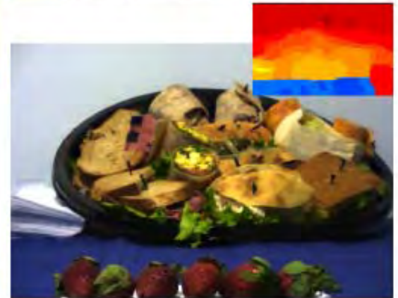
Figure 15: Partially defocused images from a standard lens, compared with an all-focused image and depth map produced by the lattice-focal lens.
