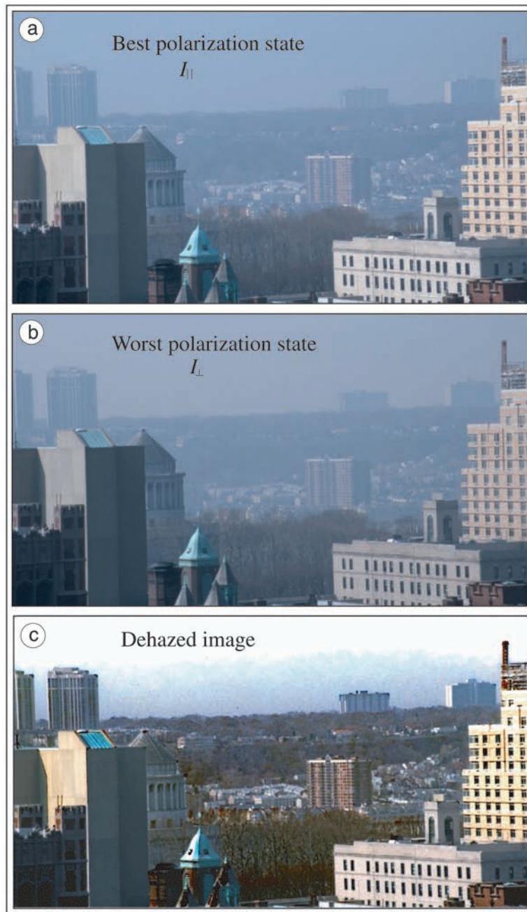
Fig. 5. Photograph with the best contrast that optics alone can give (a) is almost as poor as the worst polarization state (b). The dehazed image (c) has much better contrast and color, especially in the distant regions of the scene (note the green forest and the red roofs).
