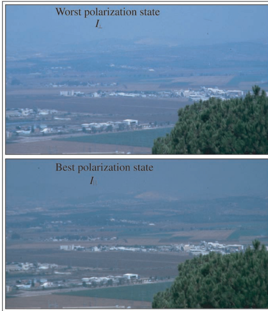
Fig. 3. Images of the polarization components corresponding to the minimal and the maximal radiances. Note that I^{\parallel} (the image of irradiance) has the best image contrast that optics alone can yield, and yet there is no significant improvement over the image of the worst polarization state.
