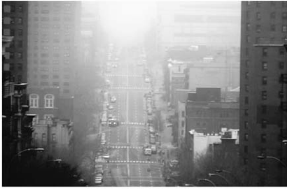
Fig. 12. Artificial contrast enhancement (not contrast restoration) of a foggy image by histogram equalization does not remove fog completely at all depths in the scene. In this example, farther depths have poorer contrast when compared to the nearer depths.
