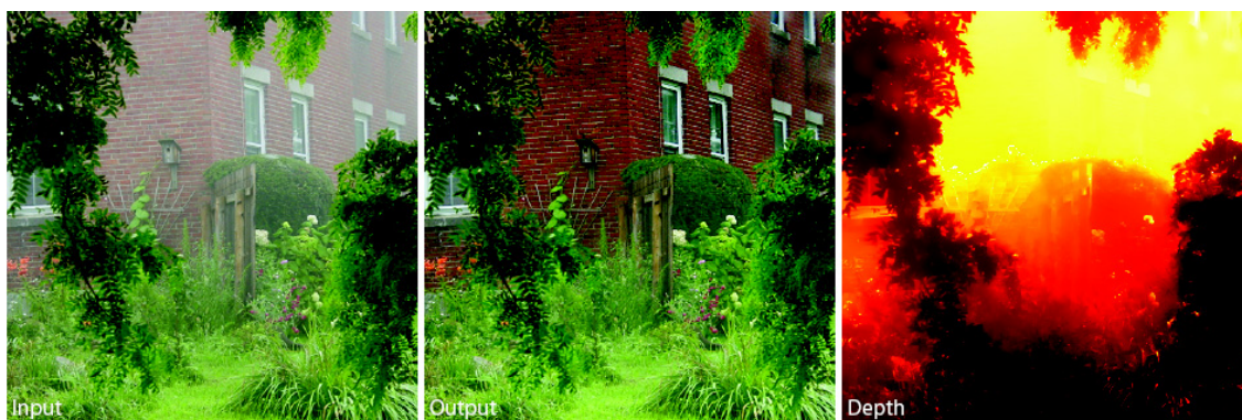
Figure 8: Dehazing based on a single input image and the corresponding depth estimate. Images taken from [1].
