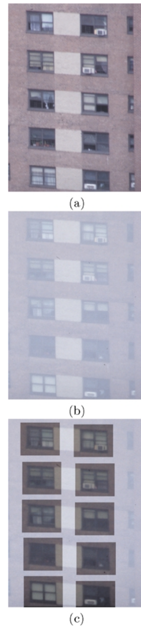
Figure 12. Demonstration of fog removal. (a) A clear day image of a building taken under an overcast sky. The color directions (and not magnitudes) of scene points (non-window regions) are recorded as true colors or clear day colors. (b) A foggy day image of the same scene again captured under an overcast sky. Note: Even though both images in (a) and (b) were taken on overcast days (i.e., spectral composition of the daylight on both days are more or less identical), the horizon brightnesses (and/or camera exposure parameters) can vary. (c) The true colors recorded were used to decompose the foggy image into direct transmission and airlight components. The airlight component was subtracted from the window regions to demonstrate a simple form of weather removal.
