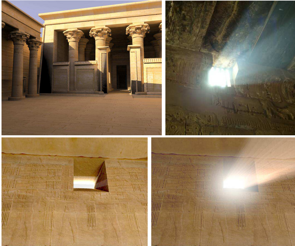
Figure 9: (top left) High-fidelity reconstruction and sun simulation of the ancient Egyptian temple of Kalabsha rendered in Radiance, (top right) photograph of volumetric light in an Egyptian temple, (bottom) visual comparison of two renderings of one interior window of the Kalabsha temple rendered in Lucifer: (left) without participating media, (right) with participating media.
