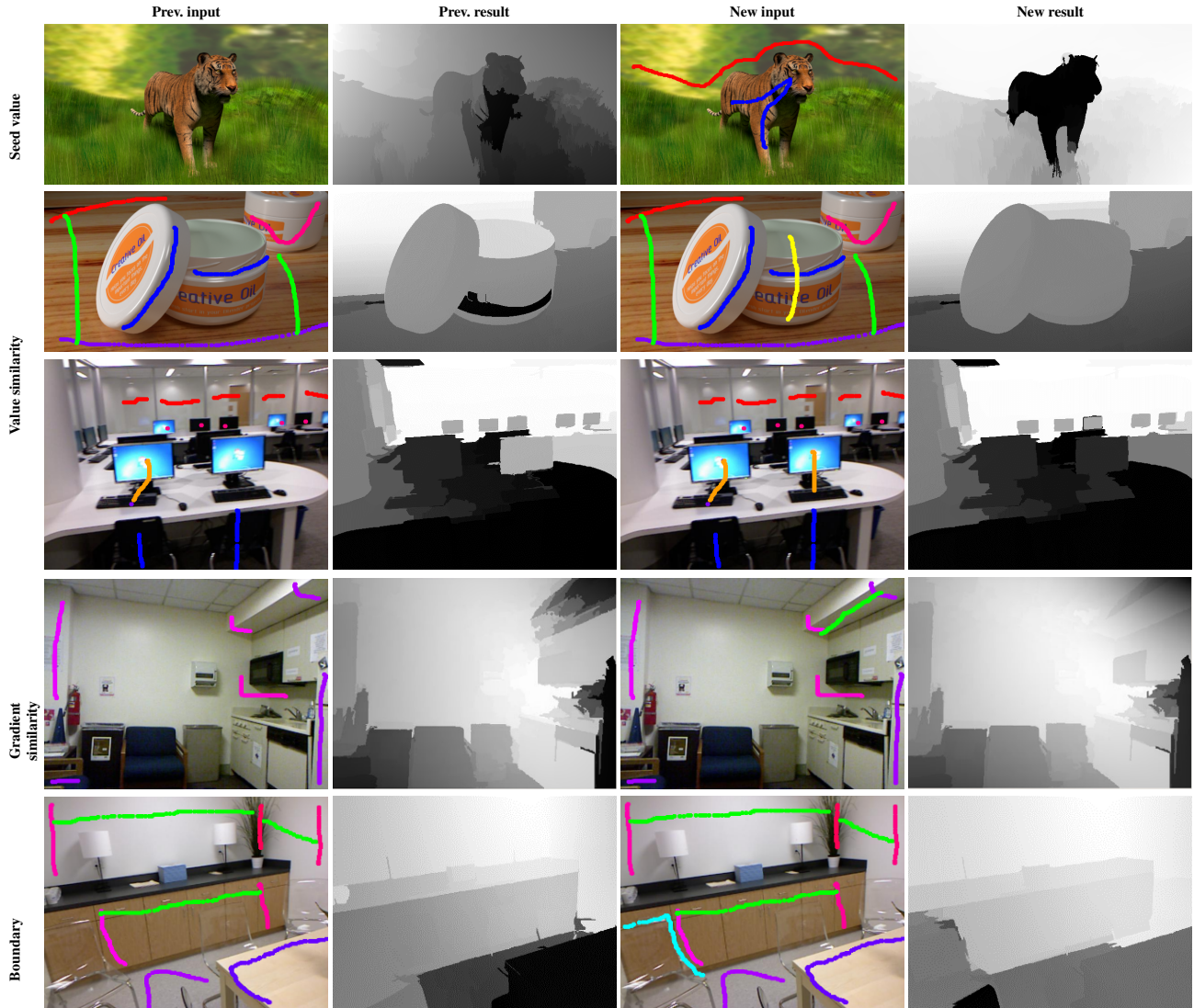
Figure 3: Individual effect of each brush with the example of depth editing. From left to right: input before the edit, depth map before the edit, new user stroke with the specific brushes, depth map after the edit. From top to bottom: seed value brushes (two strokes with different values), value similarity brush (single user stroke), value similarity brush (two separate but connected user strokes), gradient similarity brush (user stroke forces a planar surface), boundary brush (user stroke forces depth difference around the chair). Note that on each case (row) the effect of each user stroke is both meaningful and practicable.
