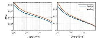
Figure 7: Convergence plots for our vector light transport (polarization) compared against traditional scalar rendering, for Figure 3 (left) and Figure 4 (right).
