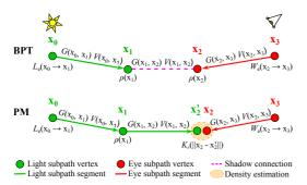
Figure 1: Schematic description of bidirectional path tracing (BPT, top) and photon mapping (PM, bottom). In both algorithms, a sensor and a light subpath are traced from the eye and the light source respectively; these two subpaths are then connected to form a full path, via deterministic shadow connection in the case of bidirectional path tracing, and via an additional random segment and density estimation in photon mapping (Figure after Georgiev et al. [GKDS12]).
