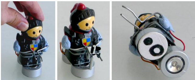
Figure 7. Hero playing piece. Left: without the Sword, the electric circuit is open. Center: placing the metal Sword between the two electric terminals closes the circuit. Right: The IR LED on the base of the toy comes on when the circuit is closed.
