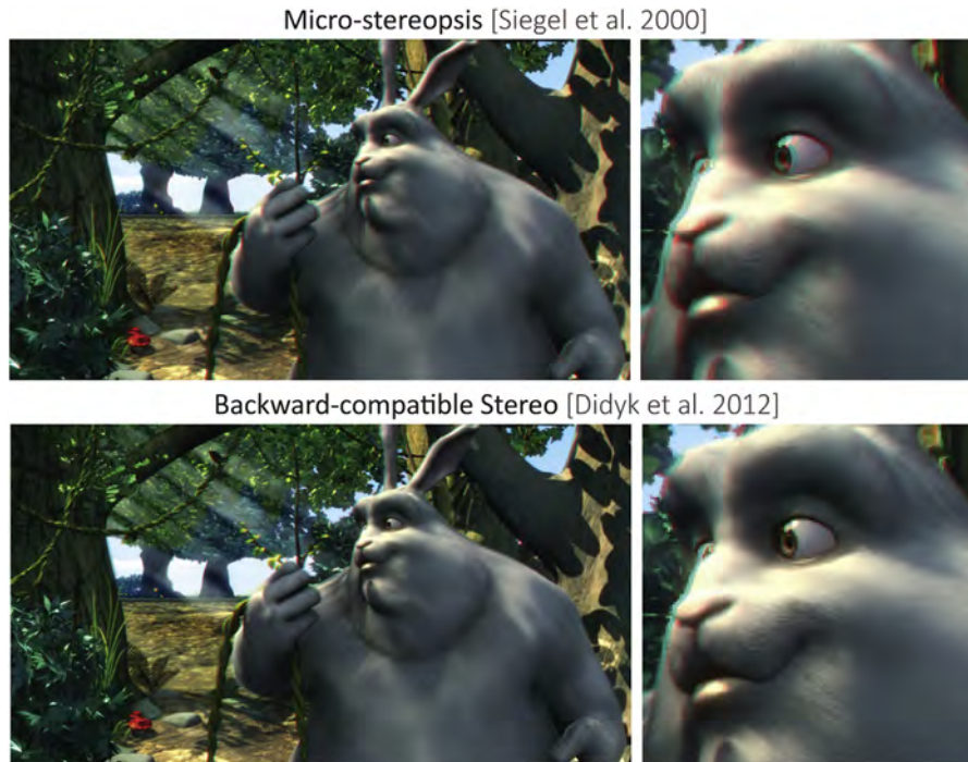
Fig. 24. Left: microstereopsis [268] reduces disparity to the minimum value that would enable 3D perception. Right: backward-compatible stereo [269] aims at preserving the perception of depth in the scene while reducing disparities to enable “standard 2D viewing” (without glasses) of the scene; the Craik–O’Brien–Cornsweet illusion for depth is leveraged in this case to enhance the impression of depth in certain areas while minimizing disparity in others (image copyright IS&T 2012).
