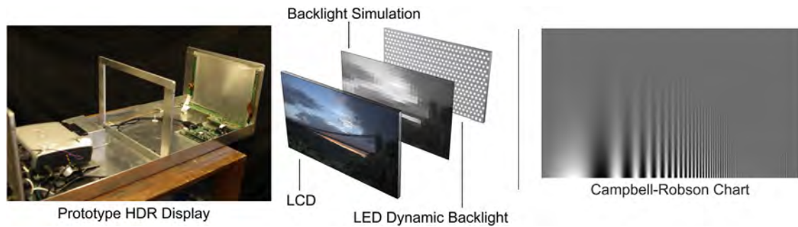
Fig. 5. Left: The first HDR prototype display, employing dual modulation (image from [34], copyright ACM 2004). Center: scheme illustrating the functioning of dual modulation, please refer to the text for details (image source: LCDTV Buying Guide). Right: the contrast sensitivity function, represented by a Campbell–Robson chart [37]; the abscissa corresponds to increasing spatial frequencies, the ordinate to decreasing amplitude of the contrast. The chart shows that the sensitivity of the HVS to contrast depends on the spatial frequency of the signal, and follows an inverted U-shape.
