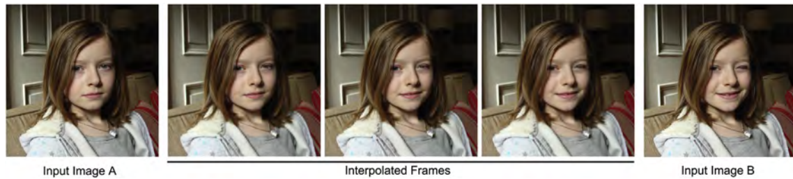
Fig. 18. Temporal upsampling: the three frames shown in the center have been synthesized from two input images, shown in the leftmost and rightmost images, by moving gradients along a path [232] (image copyright ACM 2009).
