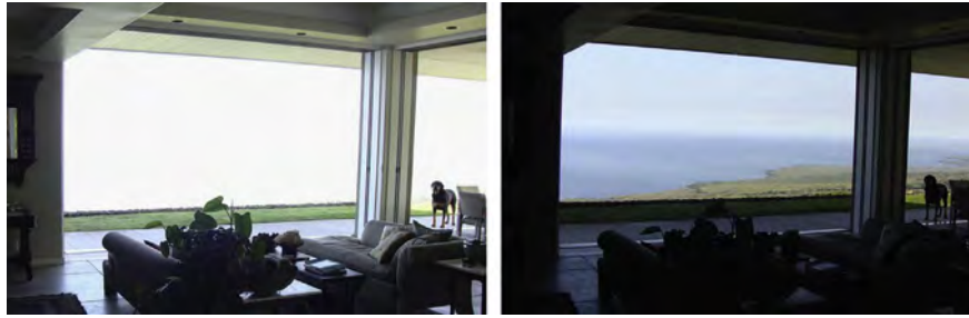
Fig. 3. Low dynamic range depictions of a high dynamic range scene, showing large saturated (left) or dark areas (right).
