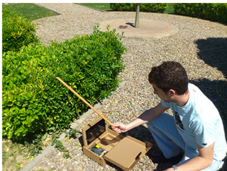
Figure 7: Setup of the mobile environment. The tablet records the movement of the shadow projected by the stick.
