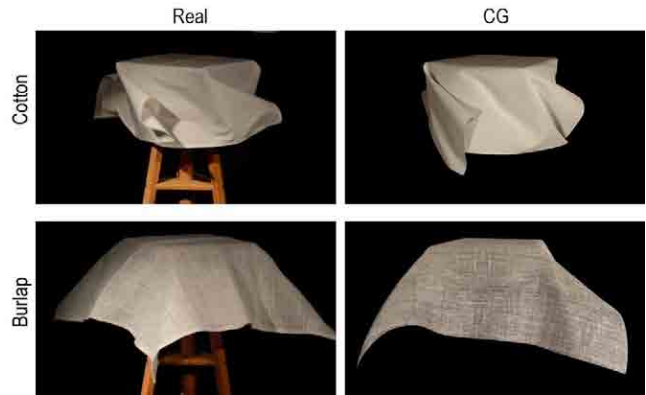
Figure 4: Comparison between the movements of the real cloth samples and the CG replicas. The first row shows the cotton rotating at the maximum speed. The second row shows the burlap at the frame just before starting to stabilize. Note that the real and CG samples are rotating in the same direction in these images just for comparison, but do so in opposite directions during the experiments to avoid exact image matching. To emulate the cloth motion, we paid special attention to the number, size and shape of the folds created (both at static and dynamic frames), the amount of bouncing, the effect of air forces, and the maximum height and width reached when rotating. For further comparisons, a selection of the videos are included in the supplementary material.
