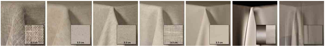
Figure 2: Comparison between the real fabrics and the CG replicas. From left to right: burlap, canvas, denim, linen, cotton, polyester satin and sheer silk. The images show renders, the insets are close up pictures of the real fabrics in the case of the first five rows. In the case of the last two fabrics on the right (polyester satin and sheer silk), the weaving pattern is too small to notice at normal viewing distances. Thus, for polyester satin the inset shows the fabric wrapping a cylinder along the warp and weft directions to show the viewing and lighting dependent anisotropic highlights. For the sheer silk, the inset shows the real fabric draping the swivel stool.
